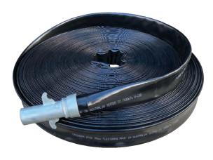
Flexidrag® is a high-quality linear move and travelling irrigator hose. It is manufactured by weaving a textile reinforcement of high-tensile polyester and encasing it with abrasion-resistant polyurethane. Our technically-advanced annealing process gives the finishing treatment to this layflat hose, making it world's best standard. Flexidrag® is able to withstand high pressures on water guns as well as remain flexible at low pressures on linear irrigators.
