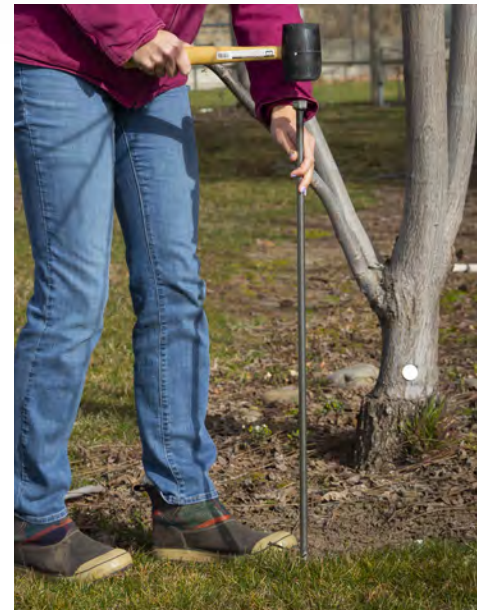
Use stake install tool 13429 to pre-make holes for the QC4 and QC5 stakes. This ensures that the stakes will be installed straight.
