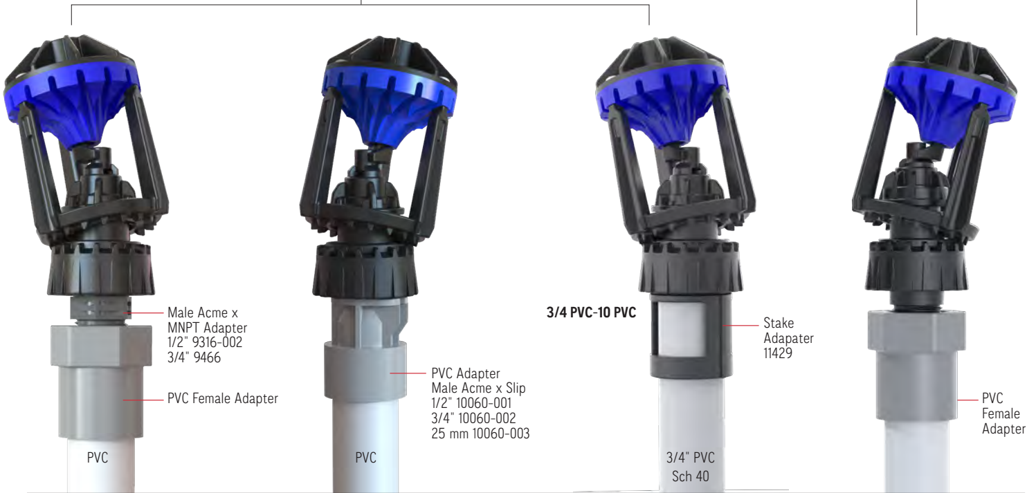
R2000FX with Female Acme connection mounts on Nelson Male Acme Adapter (shown), FT4 or FT5 Stake & Feedtube Assemblies, or options pictured below.
