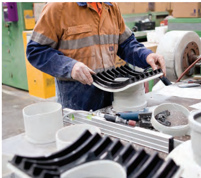
BlackMax PVC Saddle in manufacture
