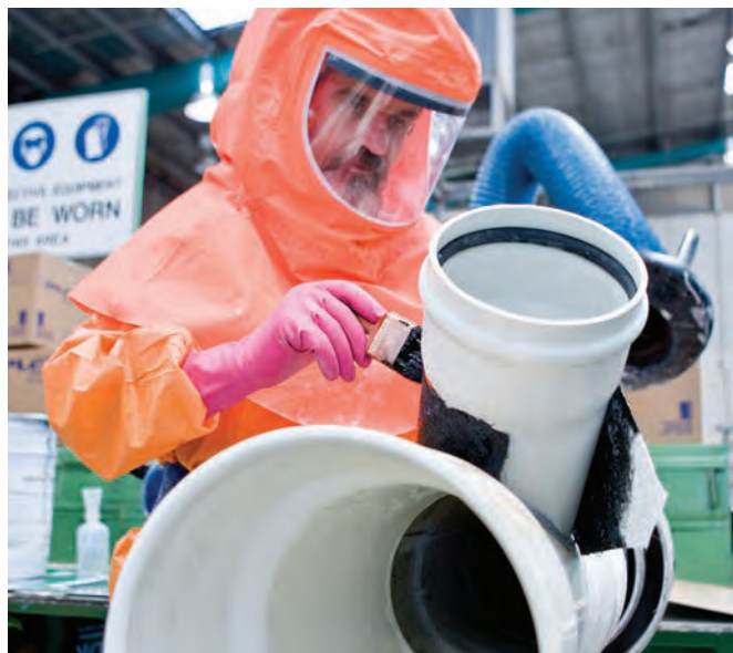
BlackMax PVC Junction in manufacture
