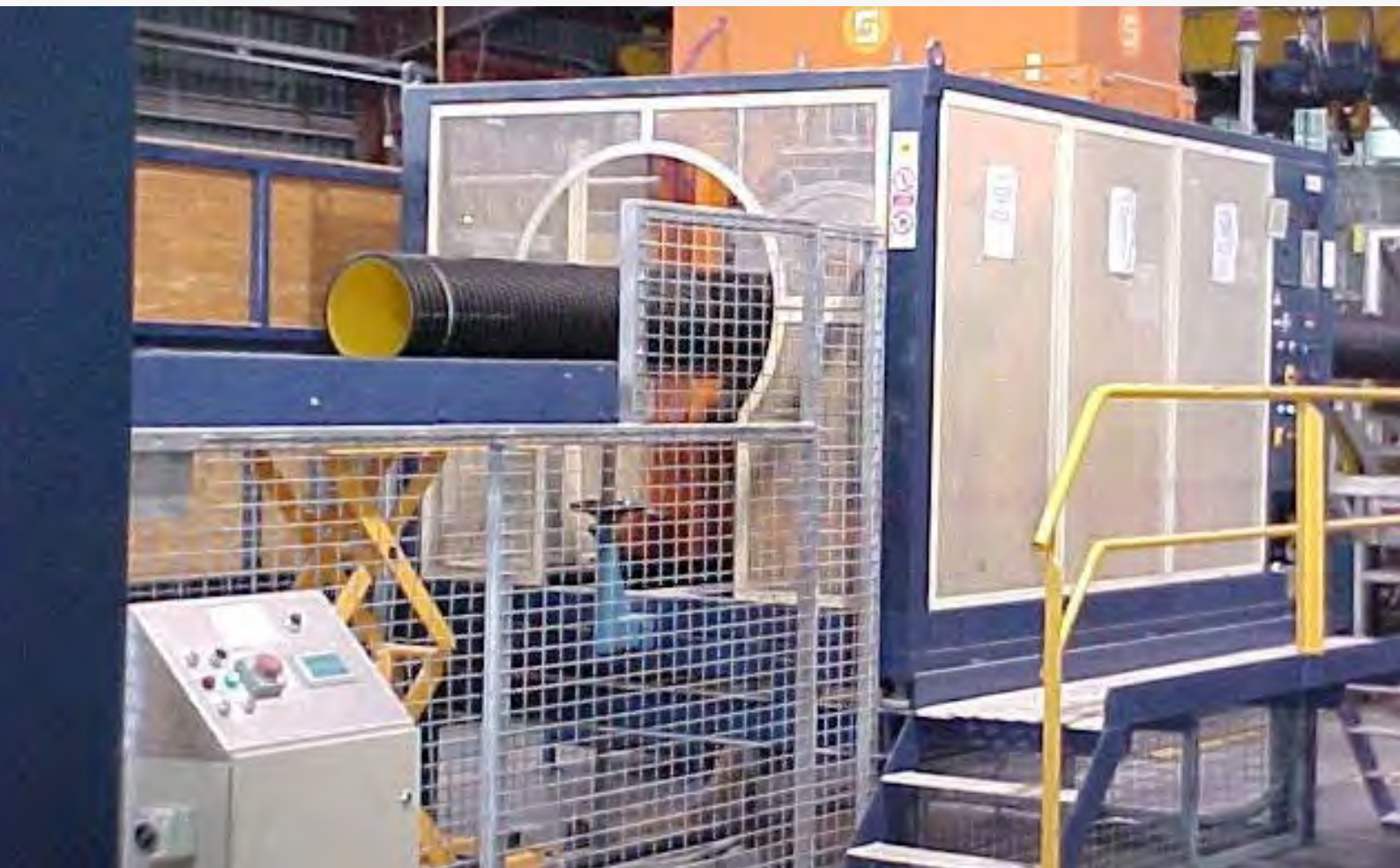
BlackMAX® pipes cut to length during manufacturing process
