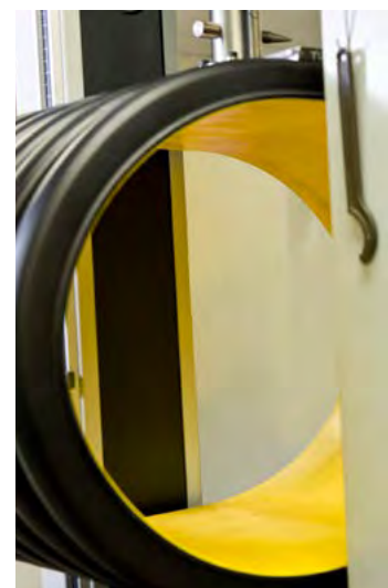
BlackMAX® PP pipe stiffness test in accordance with AS/NZS 5065
