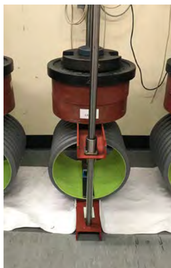
SewerMAX+® PP pipes under Creep test in accordance with ISO 9967
