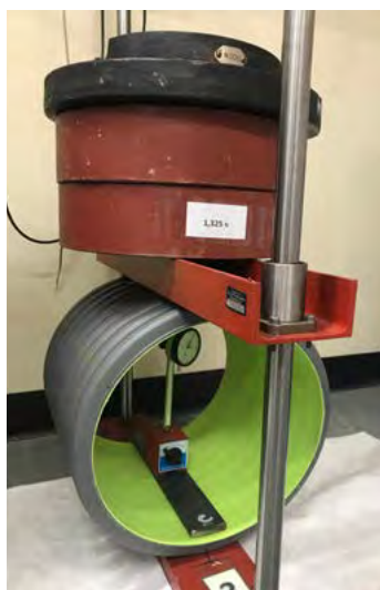
SewerMAX+® PP pipes under Creep test in accordance with ISO 9967
